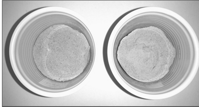
Fig.16. Soil samples: (left) Control (right) Solidified by MICP
